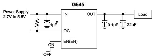
\*: 1μF of input capacitor is enough in most application cases. If the PCB trace of power rail to IN is long, larger input capacitor is necessary.
