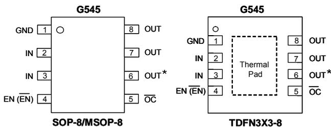
Note: Recommend connecting the Thermal Pad to the GND for excellent power dissipation.
