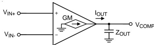
Figure 4. Operational Transconductance Amplifier, EOTA
