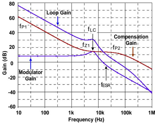
Figure 6. Typical Bode Plot of a Voltage Mode Buck Converter
