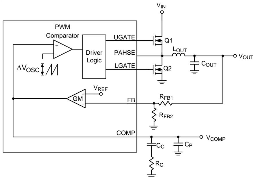
Figure 5. Typical Voltage Mode Buck Converter Control Loop
