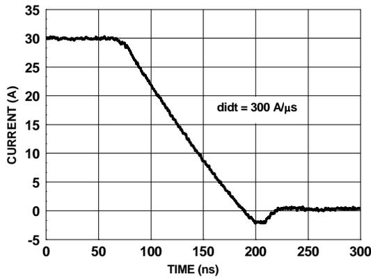
Figure 27. FDMS3600S SyncFET body diode reverse recovery characteristic
