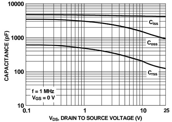
**Figure 21. Capacitance vs Drain to Source Voltage**
