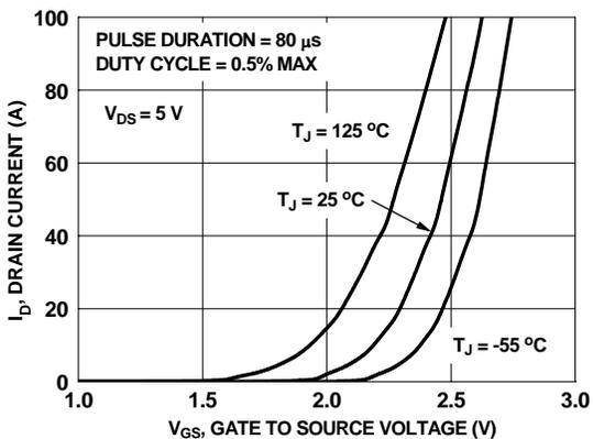
Figure 18. Transfer Characteristics
