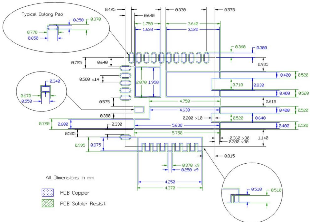
Figure 4: Solder resist
