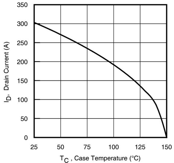
**Fig 20. Maximum Drain Current vs. Case Temperature**
