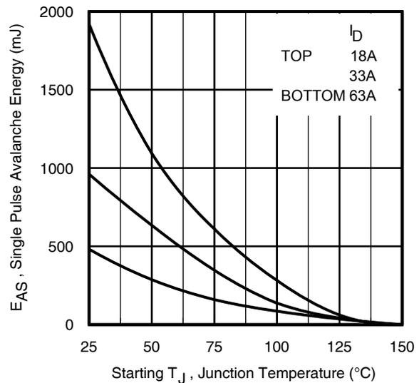
**Fig 24. Maximum Avalanche Energy vs. Drain Current**
