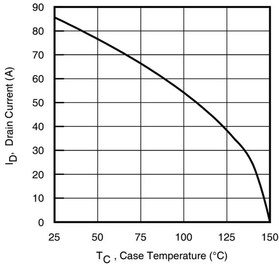
**Fig 19. Maximum Drain Current vs. Case Temperature**
