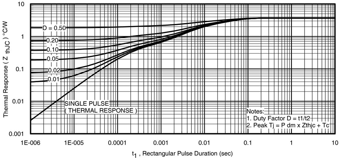
**Fig 25.** Maximum Effective Transient Thermal Impedance, Junction-to-Case (Q1)
