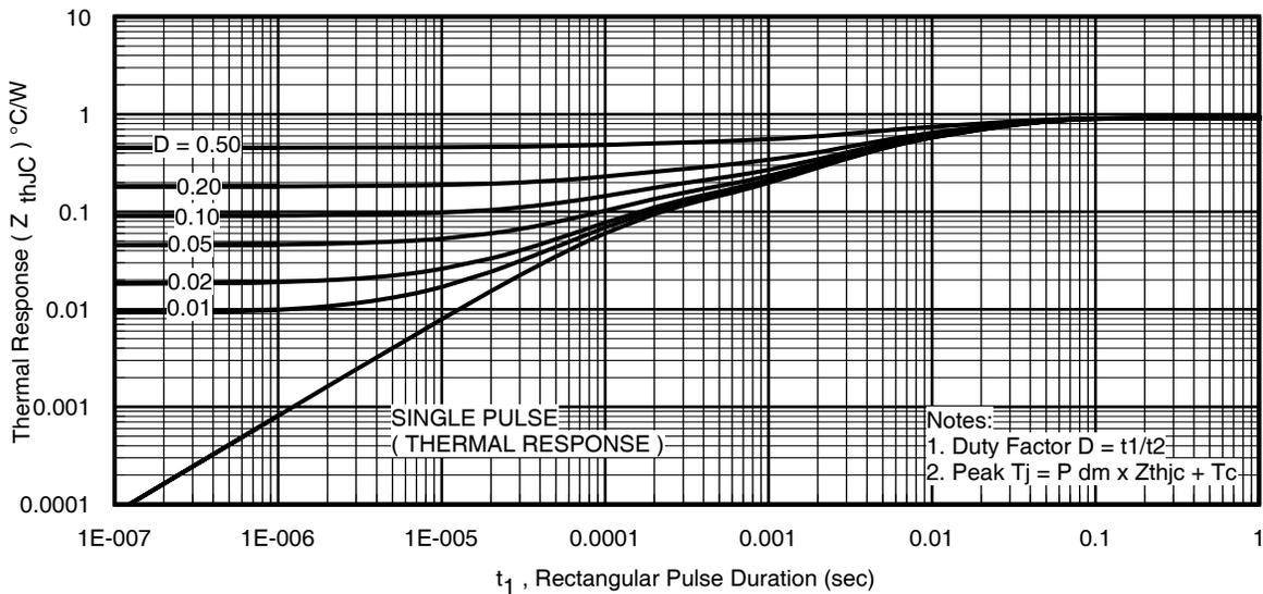
**Fig 26.** Maximum Effective Transient Thermal Impedance, Junction-to-Case (Q2)
