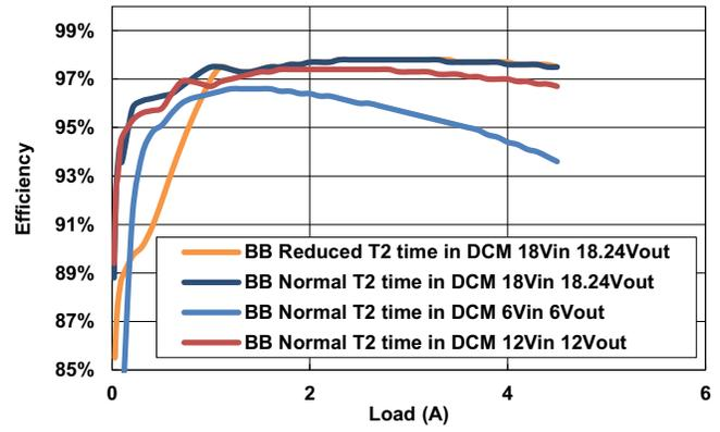
Figure 25. Buck-Boost Mode Efficiency
