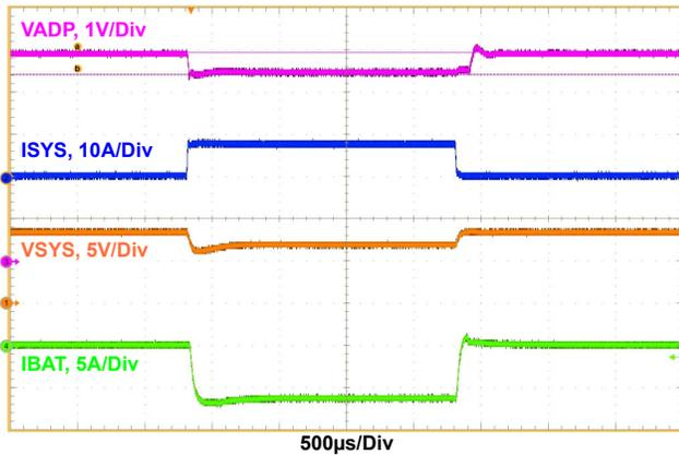
Figure 18. Boost Mode, Output Voltage Loop to Input Voltage Loop Transition,  $V_{ADP} = 5V$ ,  $V_{BAT} = 8V$ ,  $MaxSystemVoltage = 8.384V$ ,  $Charge\_current = 0A$ ,  $System\_load = 0.5A$  to  $8A$ ,  $Input\_voltage\_dac = 4.437V$
