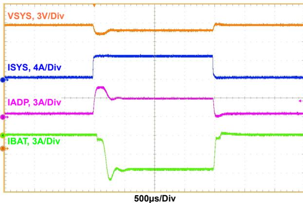
Figure 22. Bypass (HPBB) Mode, Reverse Turbo Boost Enabled. Output Voltage Loop to Adapter Current Limit Loop Transition.  $V_{ADP} = 20V$ ,  $V_{BAT} = 8V$ ,  $MaxSystemVoltage = 8.384V$ ,  $Adapter\_current\_limit = 3A$ ,  $Charge\_current = 0A$ ,  $System\_load = 0.5A$  to  $5A$
