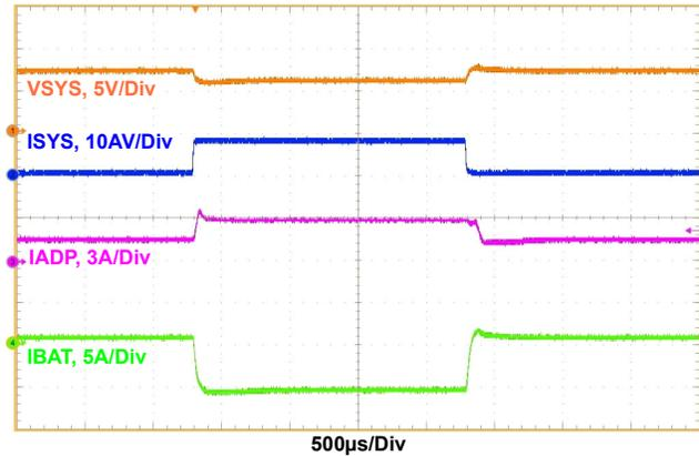
Figure 13. Boost Mode, Charge Current Loop to Adapter Current Loop Transition,  $V_{ADP} = 5V$ ,  $V_{BAT} = 7V$ ,  $MaxSystemVoltage = 8.384V$ ,  $Adapter\_current\_limit = 3A$ ,  $Charge\_current = 0.5A$ ,  $System\_load = 0.5A$  to  $8A$
