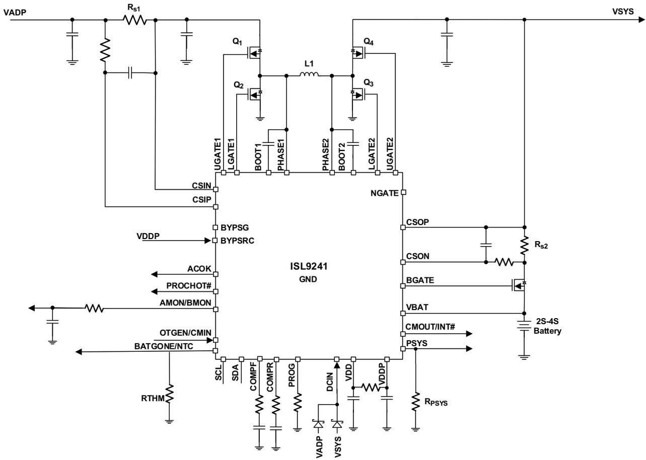
Figure 3. NVDC Only Simplified Application Diagram
