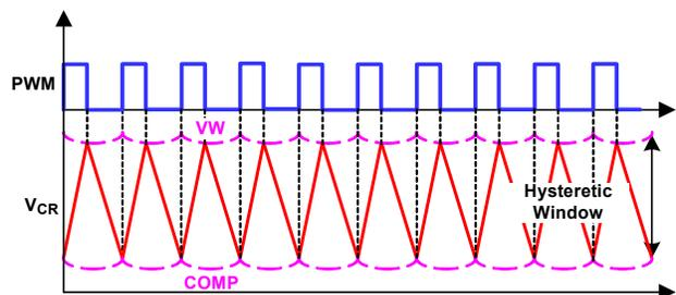
**Figure 45. R3 Modulator Operation Principles in Steady State**
