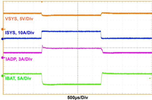
Figure 15. Buck\_Boost Mode, Charge Current Loop to Adapter Current Loop Transition,  $V_{ADP} = 9V$ ,  $V_{BAT} = 8.4V$ ,  $MaxSystemVoltage = 8.8V$ ,  $Adapter\_current\_limit = 3A$ ,  $Charge\_current = 1A$ ,  $System\_load = 0.5A$  to  $8A$
