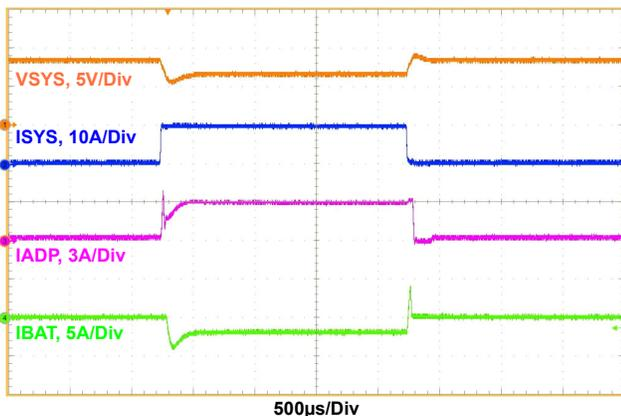
Figure 16. Buck Mode, Output Voltage Loop to Adapter Current Loop Transition,  $V_{ADP} = 20V$ ,  $V_{BAT} = 7V$ ,  $MaxSystemVoltage = 8.384V$ ,  $Adapter\_current\_limit = 3A$ ,  $Charge\_current = 0A$ ,  $System\_load = 0.5A$  to  $10A$
