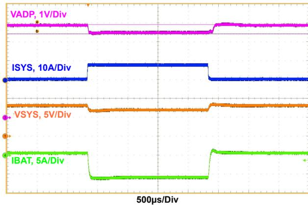
Figure 19. Boost Mode, Charge Current Loop to Input Voltage Loop Transition,  $V_{ADP} = 5V$ ,  $V_{BAT} = 8V$ ,  $MaxSystemVoltage = 8.384V$ ,  $Charge\_current = 0.5A$ ,  $System\_load = 0.5A$  to  $8A$ ,  $Input\_voltage\_dac = 4.437V$
