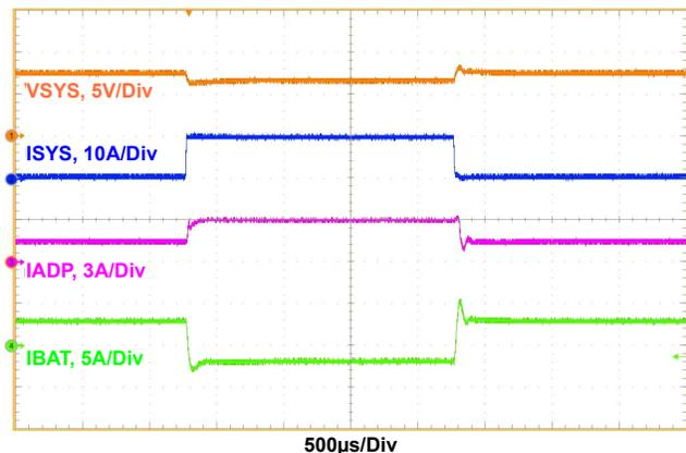
Figure 17. Buck Mode, Charge Current Loop to Adapter Current Loop Transition,  $V_{ADP} = 20V$ ,  $V_{BAT} = 7V$ ,  $MaxSystemVoltage = 8.384V$ ,  $Adapter\_current\_limit = 3A$ ,  $Charge\_current = 3A$ ,  $System\_load = 0.5A$  to  $10A$
