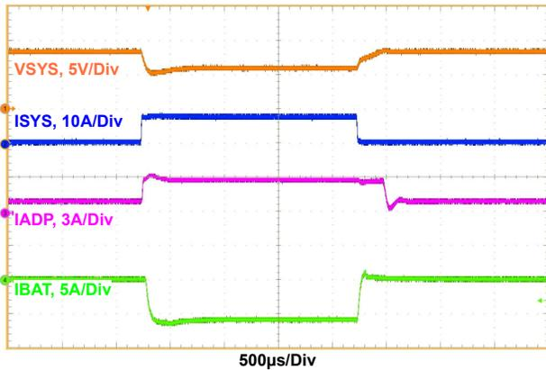
Figure 12. Boost Mode, Output Voltage Loop to Adapter Current Loop Transition,  $V_{ADP} = 5V$ ,  $V_{BAT} = 7V$ ,  $MaxSystemVoltage = 8.384V$ ,  $Adapter\_current\_limit = 3A$ ,  $Charge\_current = 0A$ ,  $System\_load = 0.5A$  to  $8A$
