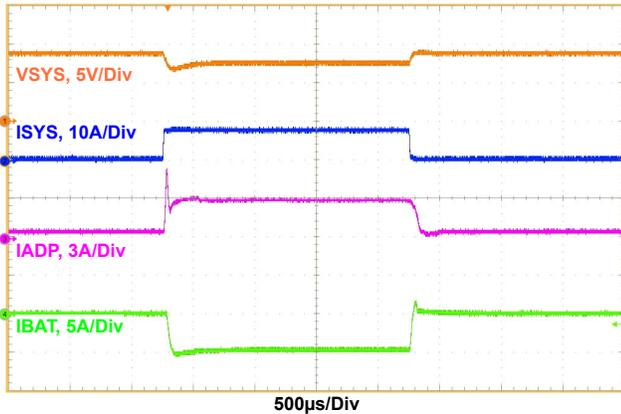
Figure 14. Buck\_Boost Mode, Output Voltage Loop to Adapter Current Loop Transition,  $V_{ADP} = 9V$ ,  $V_{BAT} = 8.4V$ ,  $MaxSystemVoltage = 8.8V$ ,  $Adapter\_current\_limit = 3A$ ,  $Charge\_current = 0A$ ,  $System\_load = 0.5A$  to  $8A$
