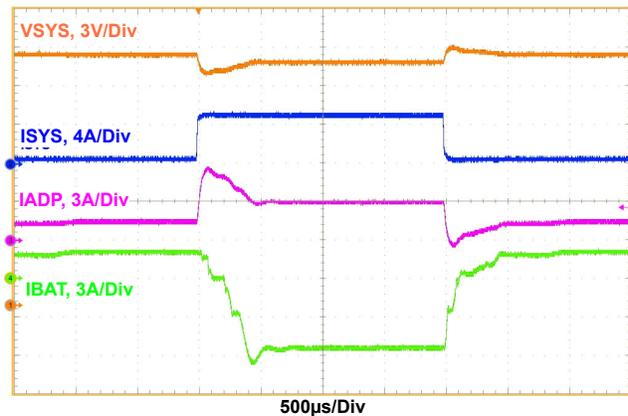
Figure 23. Bypass (HPBB) Mode, Reverse Turbo Boost Enabled. Charge Current Loop to Adapter Current Limit Loop Transition.  $V_{ADP} = 20V$ ,  $V_{BAT} = 8V$ ,  $MaxSystemVoltage = 8.384V$ ,  $Adapter\_current\_limit = 3A$ ,  $Charge\_current = 2A$ ,  $System\_load = 0.5A$  to  $5A$
