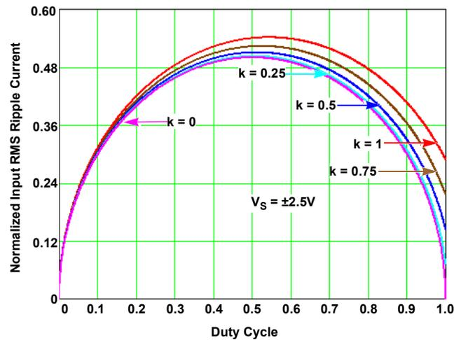
Figure 50. Normalized RMS Input Current at EFF = 1
