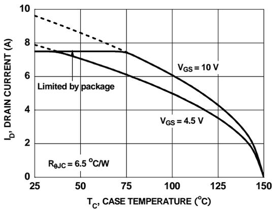
**Figure 11. Maximum Continuous Drain Current vs Case Temperature**
